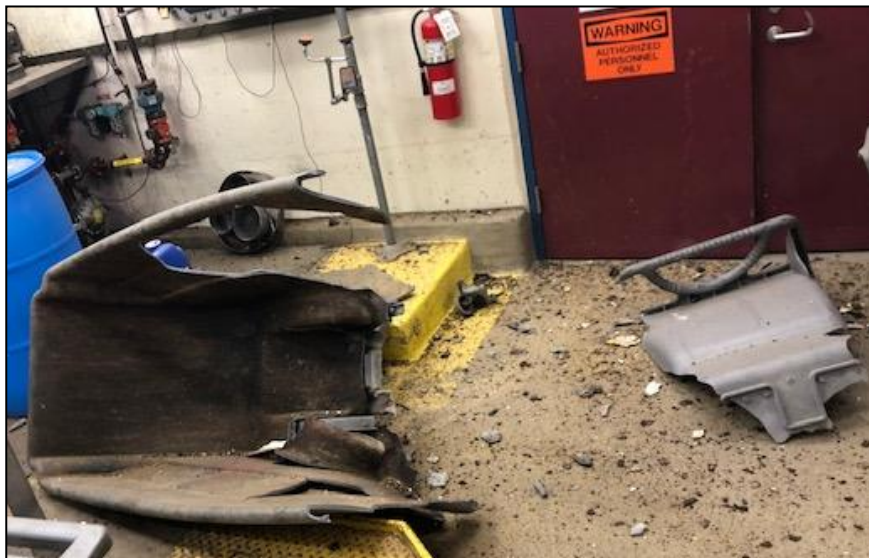
Figure 4: Damaged cart and glass fragmentation from the detonation
