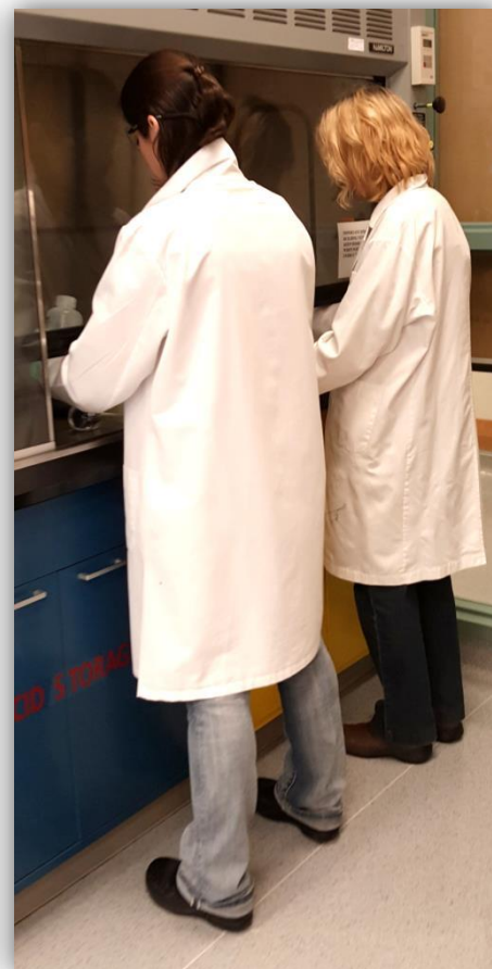
Figure 3: Some departments require extra PPE, such as lab coats, to enter the lab. Also, some lab work may require the use of additional PPE.
