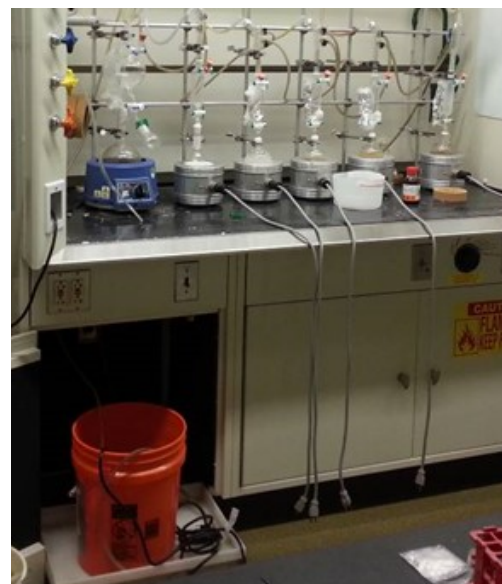
Figure 3: Solvent still system with a recirculating chiller pump in a bucket on the floor
