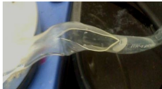
Figure 4: Split hose from a reflux condenser that flooded a lab
