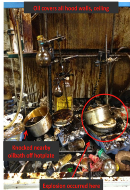
Figure 3 UMN hot plate incident hot oil sprayed all over fume hood.
