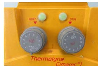
This hot plate has very similar controls for heating and stirring.
