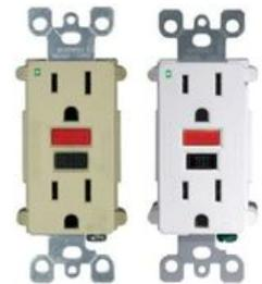
These outlets must be used anywhere that is within 6 feet of water – kitchens, bathrooms, outdoors, garages, and anywhere near a sink. GFCI outlets should be tested monthly by plugging a device into it, turning it on, and then pressing the "TEST" button on the outlet. The device should stop running as power is cut off. Extension cords with a GFCI built in are also available. These are good to use in damp or wet areas.
