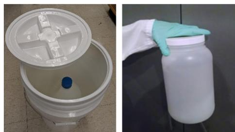
Figure 2: Transport of hazardous chemicals outside of the lab
