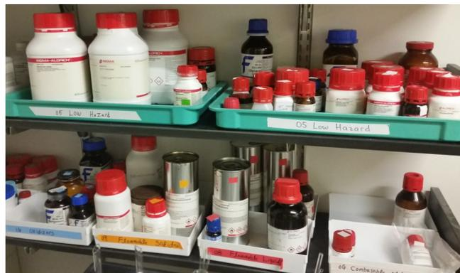
Figure 1: Storage bins used to segregate different hazard classes
