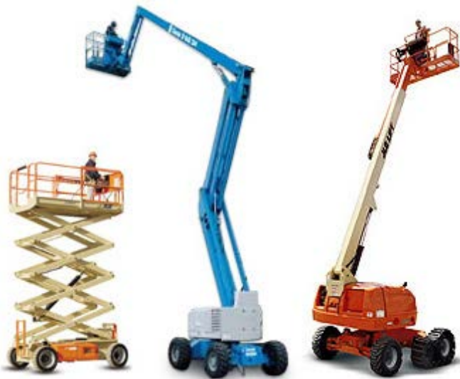
Figure 1. Common types of aerial lifts. Left: vertical only/scissor lift. Center: articulating boom lift. Right: telescoping boom lift.
